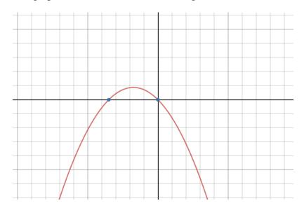
Here, f(y) is the vertical axis, y is the horizontal axis, and the blue points are the two equilibria.
