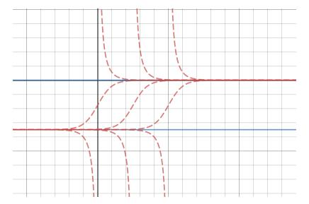
The vertical axis is y, and the horizontal axis is t. The solid blue lines are the equilibrium solutions, and the dashed red lines are the non-equilibrium solutions.
